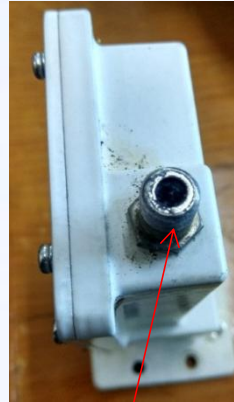
Center pin broken
